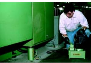
The problem was to reposition machine centers without disrupting production. "Using Simplex RLR Series cylinders and a PE70 series **Suc-O-Matic** pump, we rearranged our shop floor in one day." The low closed height and longer strokes eliminated extra jacking & blocking procedures, and the Simplex Suc-O-Matic retracted load return cylinders effortlessly.
