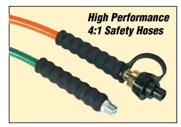
Thermo-Plastic HP & HPC Series Hoses are recommended for demanding applications. Along with their distinctive green color, the HP & HPC series hoses boast a 10,000 psi working, 40,000 psi minimum burst, (4:1 safety factor) and a tough polyurethane outer cover that resists abrasion and wear. Well suited for continuous duty, the reinforced polyester and carbon steel wire design contributes to low volume expansion, minimized fatigue and enhanced system efficiencies.
