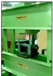
A machine shop needed to straighten forgings prior to machining. "We needed a pressing force of 100 tons and we didn't want to cut corners when it came to safety. Simplex presses do not rely on "bolt together" construction. Heavy duty pins, plus strong, welded construction across the upper bolster, puts the strength where it needs to be."
