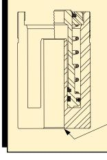
A **one piece**, **unified body** is significantly stronger than standard hollow cylinders. Special manufacturing eliminates potential leak points at the base, enhancing the integrity & alignment of the base and center tube.
