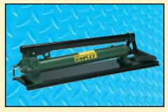
2 Speed Foot Pump: Great for hands free operation. Spring loaded release valve and pump handle allows the operator to advance, hold and release the load all by foot.
