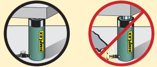
Never attempt to disconnect hydraulic hoses, fittings or couplers under pressure. Unload the ram, open the release screw on the hand pump and shift or open all hydraulic controls several times. If system includes a gauge, double check the gauge to insure pressure has been completely released.
