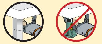
Hydraulic rams are not meant to be used as permanent supports. They are designed to lift and lower. If you need to hold the load for any length of time, cribbing or Simplex locknut cylinders should be used.
