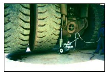
■ When It Comes To Brute Force In a Roll Under Jack, nothing even comes close to the Simplex Pow'r-Riser II<sup>TM</sup>. With capacities up to 200 tons and powered by standard shop air or 115VAC, the Simplex Pow'r-Riser II<sup>TM</sup> is ideal for the largest maintenance jobs. From the heaviest railcar to the largest mining equipment, Pow'r-Riser II<sup>TM</sup> is the only choice.
