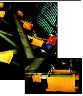
A heavy steel fabricator uses Simplex RDA10012 double acting cylinders to form large sections of I-beam. "The Simplex cylinders and pumps allow us to bend the beams to precise radiuses."
