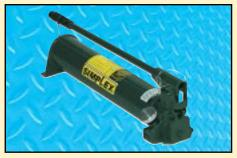
Progressive Force Hand Pump: Delivers high volume of oil up to a crossover pressure of 3,000 PSI. Model (P140F & P140DF) are faster and require less handle strokes for applications where force increases steadily throughout the cylinder stroke, such as bending, squeezing or crimping.
