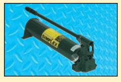
Two-Speed Hand Pump: With the cylinder unloaded, pump delivers a high volume of oil for fast cylinder speed. Once the load is engaged, the pump automatically switches to the high pressure stage.
