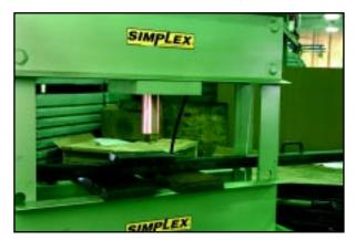
Repair personnel were faced with a variety of difficult bending, pressing, straightening and disassembly jobs. "Almost every day we have to remove bearings, straighten cylinder rods, perform wheel repair, and rebuild gear boxes. The 55 ton press is perfect; it's adjustable bed and moveable work head gives us the flexibility to work on a wide variety of jobs."
