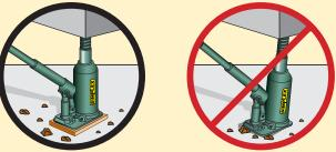
Every jack or ram, whether used individually or in a system, should be completely supported on a solid, firm, non-sliding foundation capable of supporting the load.
