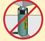
The load must be centered on the ram, or equally distributed on multiple rams. Off center loading can result in the ram slipping out and loss of the load.
