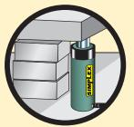
Place blocking or cribbing under the loads as you raise it. Each time you raise it higher, insert more blocking. Position yourself in a manner that will keep you clear of the load, and will not allow your hands or other body parts between the load and the cribbing.
