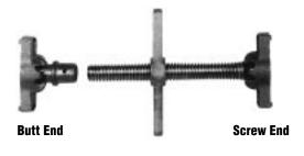
Simplex Trench Braces provide efficient, economical protection against cave-ins and costly redigging in construction and utility maintenance. Braces extend by turning the lever nut handle. The ball socket joints tilt for **added safety on angular mounting.** Holes on each end facilitate mounting to wood members.
