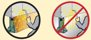
Weld splatter will damage plunger rods and hoses. Hydraulic fluid can ignite if vaporized or exposed to high temperatures.
