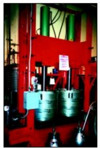
■ Choose double-acting cylinders for higher cycle production work or when complete control of larger cylinders is desired. Here two RDA-Series 150 ton cylinders are used in this custom made press to extract vanilla. "With these Simplex cylinders we can extract 30% more vanilla in less time making the process more efficient and profitable." See pages 28 - 29.
