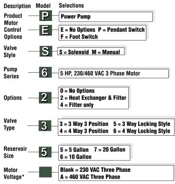
\*460 VAC pump ordered with heat exchanger requires a separate 115 VAC power source for the heat exchanger.
