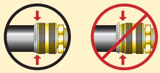
When making connections with quick couplers, make sure the couplings are fully engaged. Threaded connections such as fittings, gauges, etc. must be securely tightened and leak free. Never use excessive tightening force that may distort the fittings or strip the thread profile.
