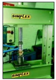
A manufacturer of industrial gear boxes used the Simplex 25 ton press in their production assembly line to press various size bearings on gear assemblies. "We can press up to 100 bearings an hour with the Simplex press. The hydraulics are reliable and easy to use and they keep working day after day."
