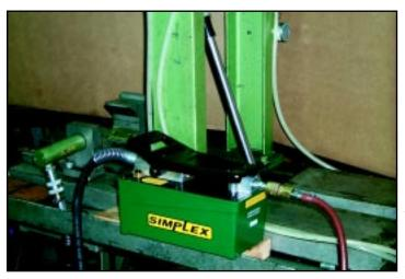
When reliable 10,000 psi power was needed to run this production line fixture, industrial engineers chose the Simplex PA91. "The three position treadle is easy to use and the pump runs on standard shop air."
