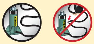
Do not drop sharp or heavy objects on hose. Keep hose out of heavy traffic areas. This will cause internal damage to hose wire strands. Applying pressure to a damaged hose may cause it to rupture. Avoid sharp bends and kinks when routing hydraulic hoses.
