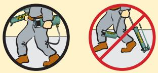
Dragging or carrying rams or pumps by a connected hose can damage the couplers and hoses. Using damaged couplers and hoses can be dangerous.
