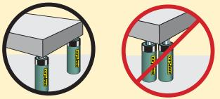
For multiple ram lifts, you must be able to determine the location and number of lifting points that will allow the load to be evenly distributed to all the rams. This is called load balance. Size, center of gravity, and load geometry must to be considered in order to correctly determine load balance.
