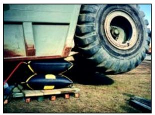
Two 72.3 ton capacity air bags are used for tire maintenance and axle inspection on off-road mining equipment.
