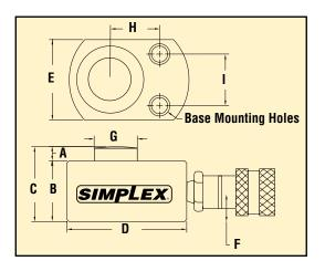
Simplex RF & RFS Series are designed specifically for near impossible lifting, clamping or positioning jobs where space is at a premium. Ideal for break loose or start up spreading jobs. These mini-monsters pack up to 150 tons of force into a convenient, portable package.
