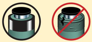
Check each component before you set up your hydraulic system. Do not use damaged or worn components. Turn them in for repair or replacement.
