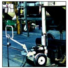
■ For Portable, Self-Contained Jacks, Nothing Beats the Simplex Pow'r-Riser II<sup>TM</sup> Railcar Jack. While short enough to fit under the lowest loads, operators can add up to 32" of drop in extenders for maximum flexibility. Dual hydraulic locking systems and mechanical lock rings make the Pow'r-Riser II<sup>TM</sup> the safest jack available.
