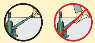
Do not use extensions or cheeter bars on hydraulic jacks or hand pumps to raise a load.
