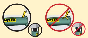
Only fill pump to recommended level, and fill only when connected cylinder is fully retracted.
