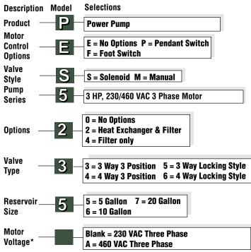
\*460 VAC pump ordered with heat exchanger requires a separate 115 VAC power source for the heat exchanger.
